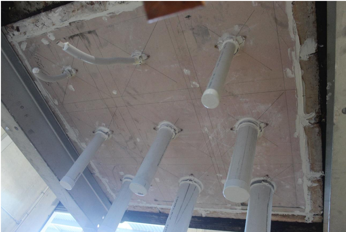
Figure 21 – Exposed face prior to test commencement
